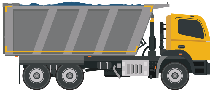
Box Capacity: 22 Cu.m, Wheelbase: 4875mm
